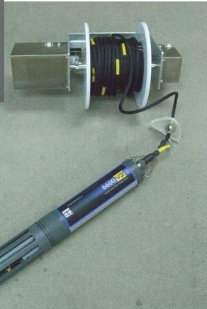
✓ **High availability.** All mechanical moving parts are designed within the modular winch head. It is common that some usage wear and tear on moving parts are inevitable. With modular winch head design any mechanical related repair or maintenance can be carried out by quick hot-swapping to the alternate winch head, thus greatly minimizing any down-time.
