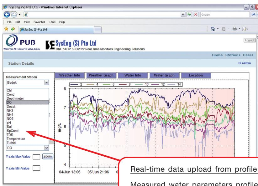
Derived water parameters profile: **DO saturation, NH<sub>3</sub>, Salinity, TDS.**
